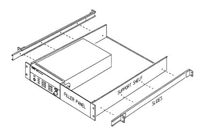
To install one or two instruments in a sliding support shelf, order shelf 5063-9255, and slide kit 1494-0015 (for single instrument, also order filler panel 5002-3999).
