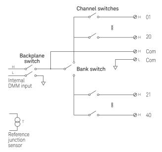
Note: Thermocouples must be electrically isolated from each other to avoid current loops and subsequent measurement errors.
