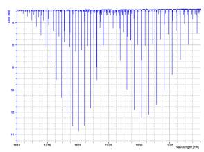
Figure 3: Absorption lines of a C<sub>2</sub>H<sub>2</sub> gas cell acquired at 200 nm/s sweep speed with the 81606A tunable laser.
