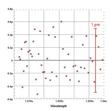
Figure 4: Less than ± 1 pm deviation of the measured center wavelengths from the known values according to NIST.
