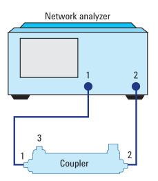
Figure 10. Equipment setup using network analyzerwith coupler
