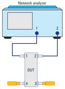
Figure 13. Equipment setup using network analyzer with coupler
