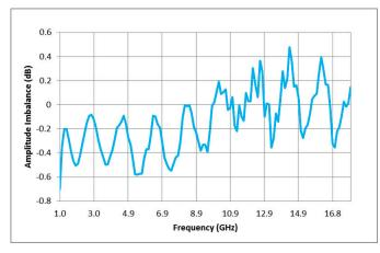
Figure 15. This graph shows the maximum deviation from 0.0 dB reference is approximately –0.7 dB at 1 GHz.
