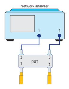
Figure 17. Equipment setup using network analyzer with coupler port 1 and port 3
