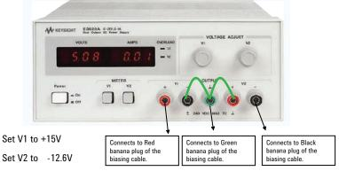
Connect V1-, GND and V2+ together as shown in above green wires.
