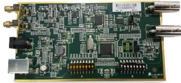
Figure 12. The Keysight AE6950A frequency divider board is used for the distortion test with disturbing signal to synchronize references of an oscilloscope and a function generator with a transmitter clock.
