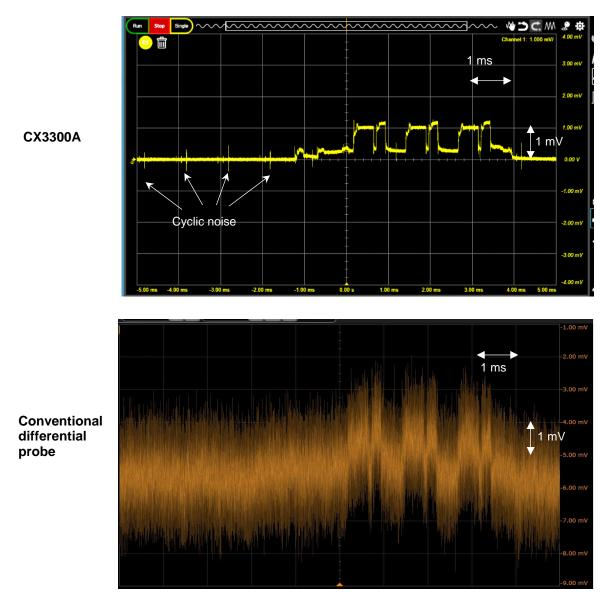
Figure 4. CX3300 captures very small differential voltage beyond a conventional differential probe
