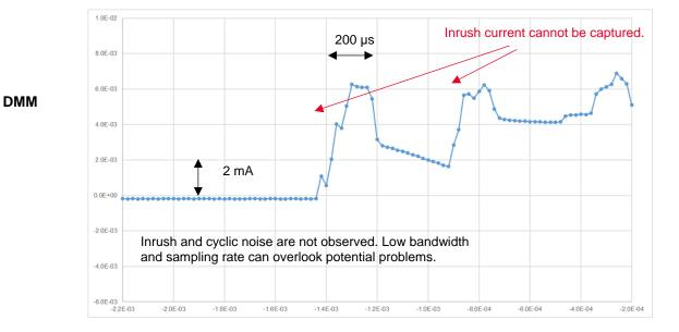
Figure 5. CX3300 captures small dynamic current and voltage signals that are not captured by a DMM
