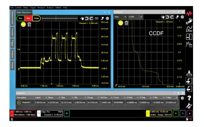
CX3300 features statistical analyses such as complementary cumulative distribution function (CCDF) or histogram on the mainframe. As a result, you can now focus on your measurement without transferring the data to your PC.
