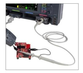
Figure 14. CX1151A passive probe interface adapter
