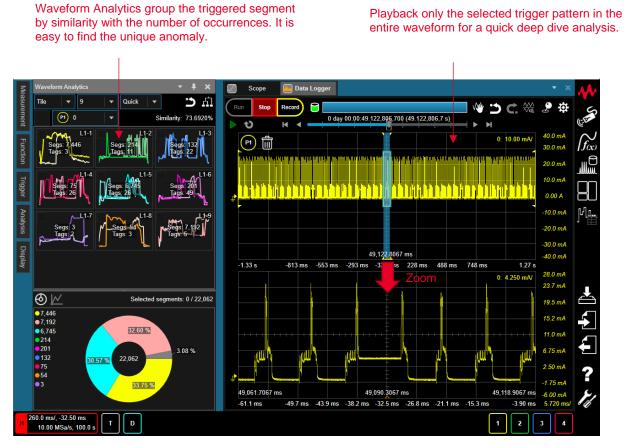
Figure 20. Waveform Analytics enables you to identify anomalies quickly
