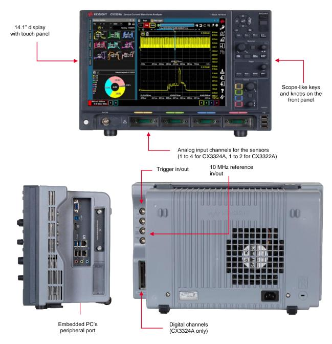
Figure 7. CX3324A front, side, and rear instrument views
