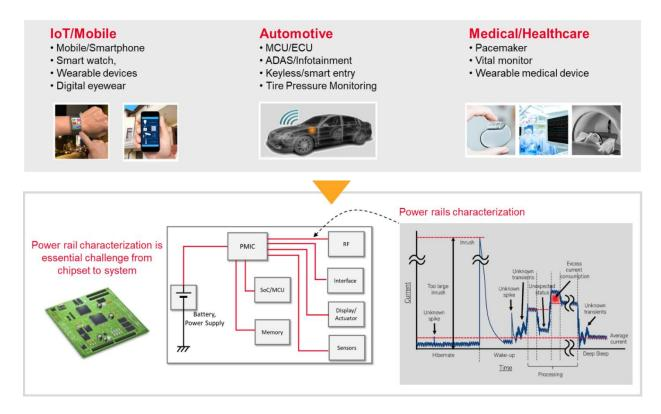
Figure 1. Power rail characterization from chipset to system
