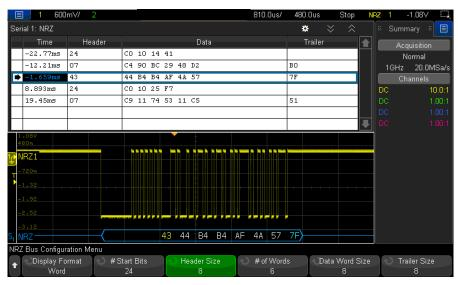
Figure 8. User-definable NRZ decode on an InfiniiVision X-Series oscilloscope.
