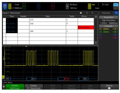
Figure 7. PSI5 decode on an InfiniiVision X-Series oscilloscope.
