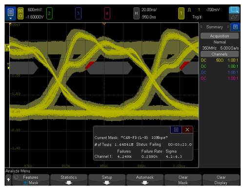
Figure 10. CAN FD eye-diagram mask testing.
