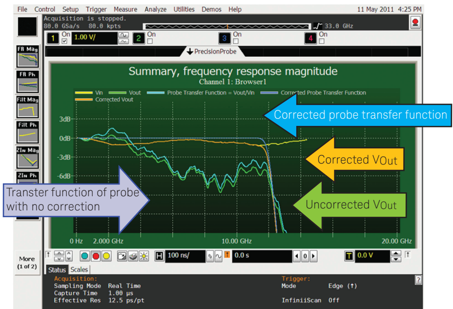
Figure 8. Notice the differences in the frequency response magnitude after the PrecisionProbe correction.
