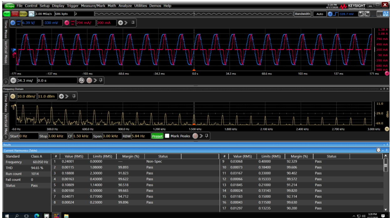
Figure 3. Current harmonics measurement based on IEC 61000-3-2 standards
