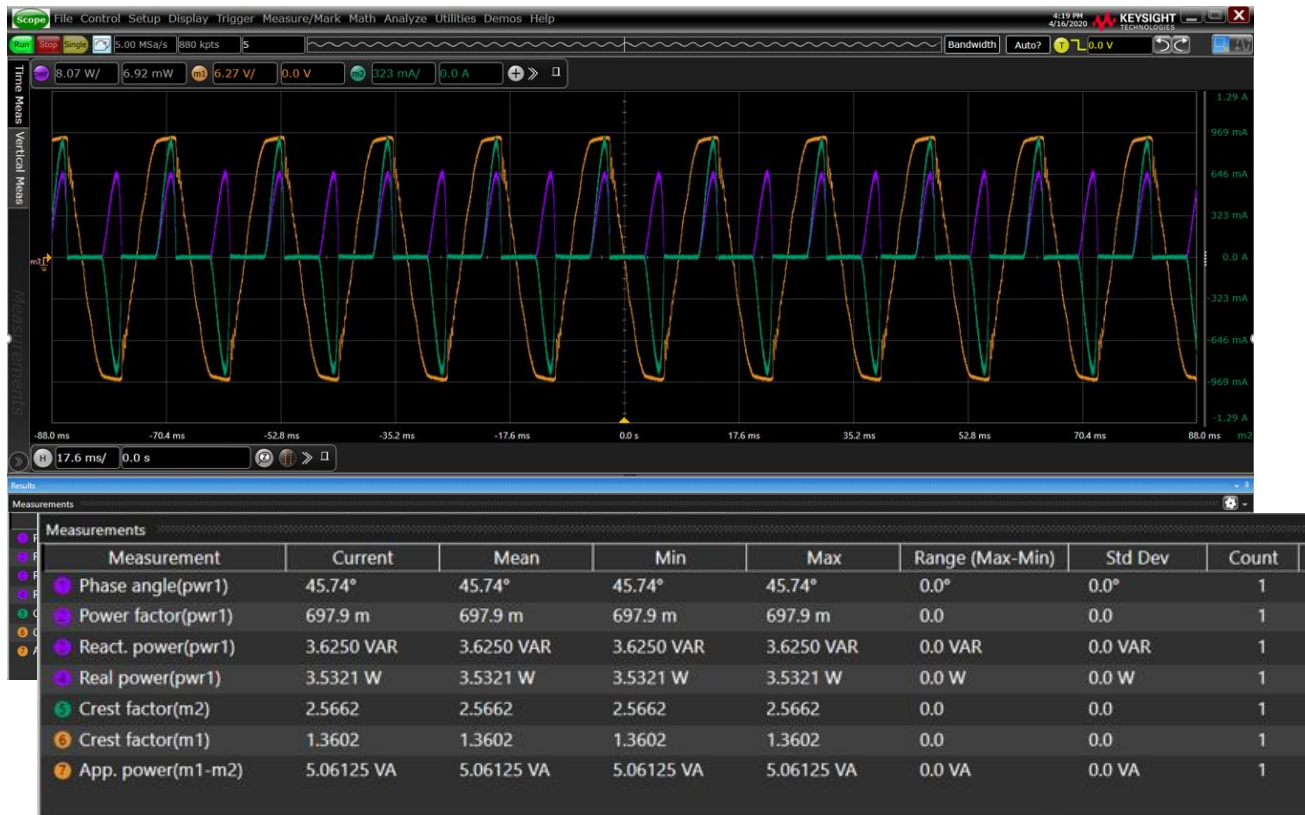
Figure 2. Input power quality measurements
