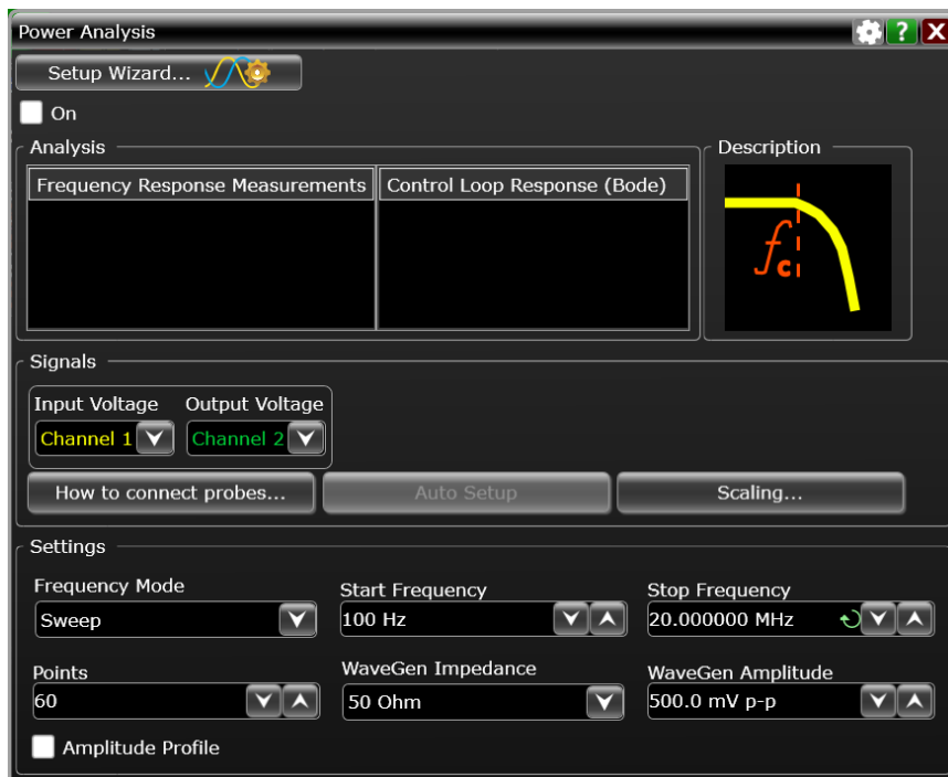
Figure 11. Frequency Response Analysis is included with the WaveGen (MXR2WAV) option in addition to the Power Supply Analysis software
