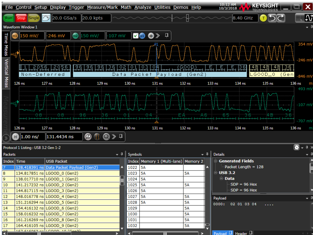
Figure 3. USB 3.2 SuperSpeed+ trigger and decode, with protocol lister and detailed packet view.
