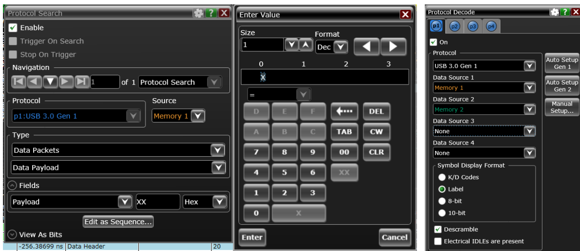
Figure 4: On the left is a comprehensive search system with a hex payload editor. On the right is the setup window.
