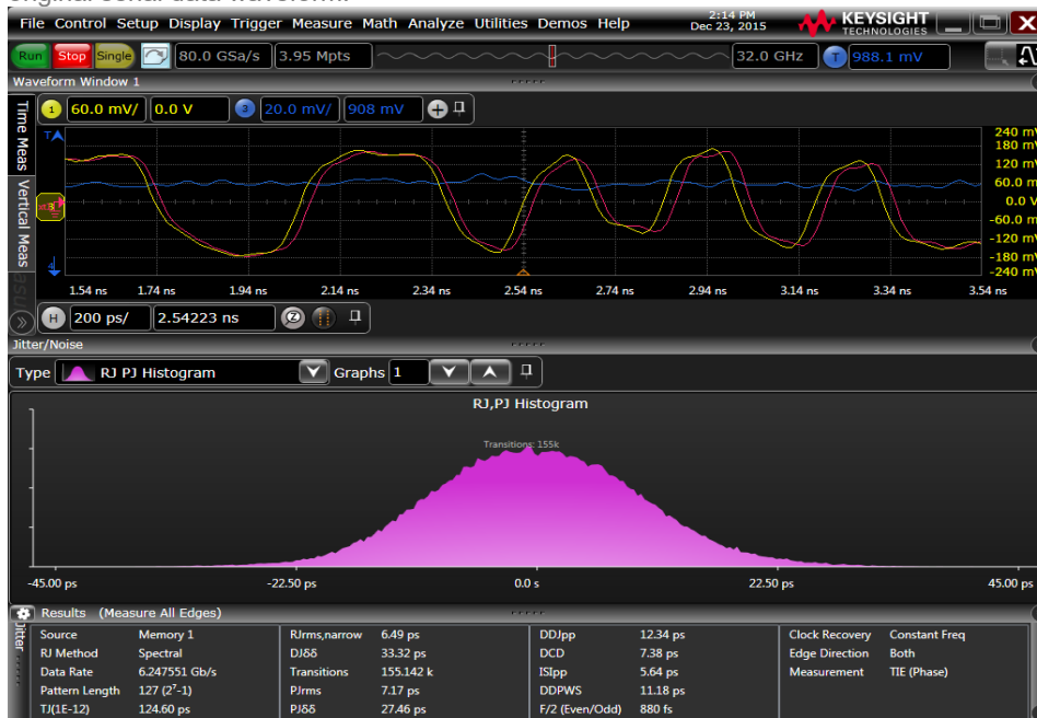
Figure 13. Jitter analysis results using EZJIT, demonstrating the improvement in jitter statistics after removing the jitter generated by the power supply.
