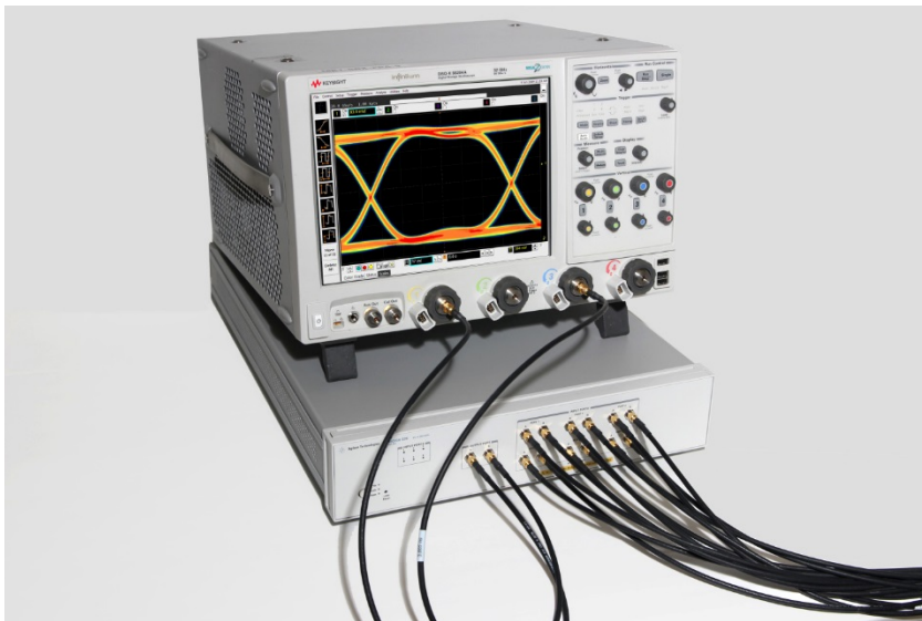
Figure 17. Automated testing for multi-lane digital bus interface through switching solution.
