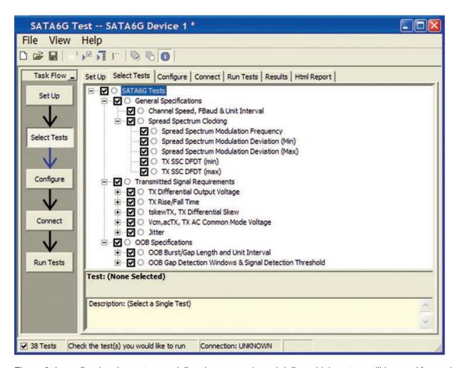
Figure 3: In configuring the tests, you define the test mode and define which pattern will be used for each test.
