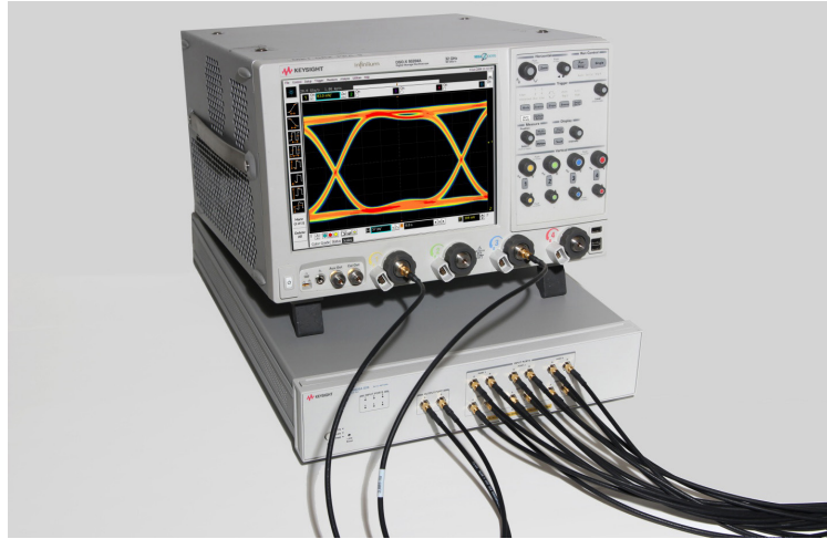
Figure 18. Automated testing for multi-lane digital bus interface through switching solution
