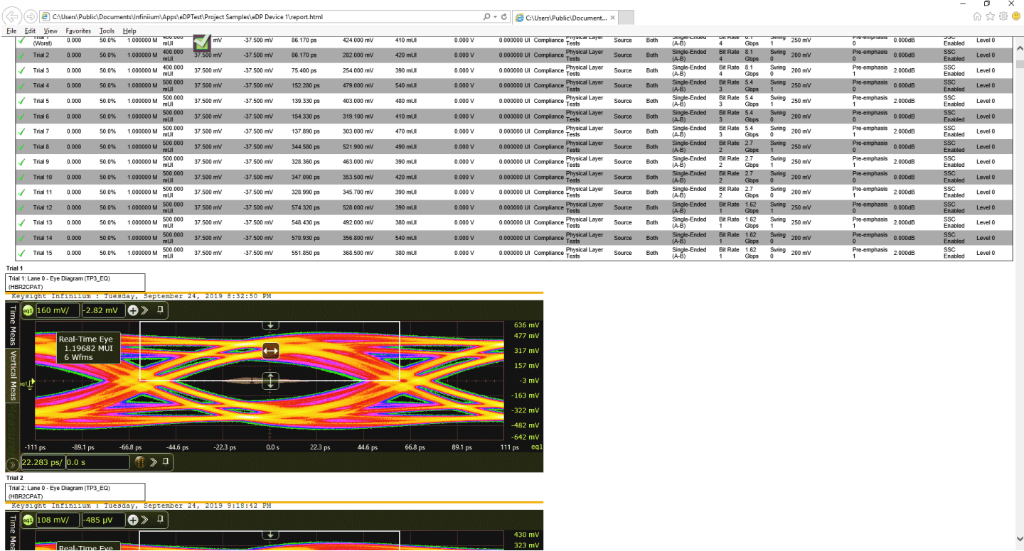
Figure 12. Summary report detail: The eDP software’s summary report provides screen shots of all the measurements that have been performed. In this figure, you can see that many data-eye measurements were made (15 trials) and the first trial screen shot is shown. Observe the clear status and description at the top and the measurement data just above the eye.
