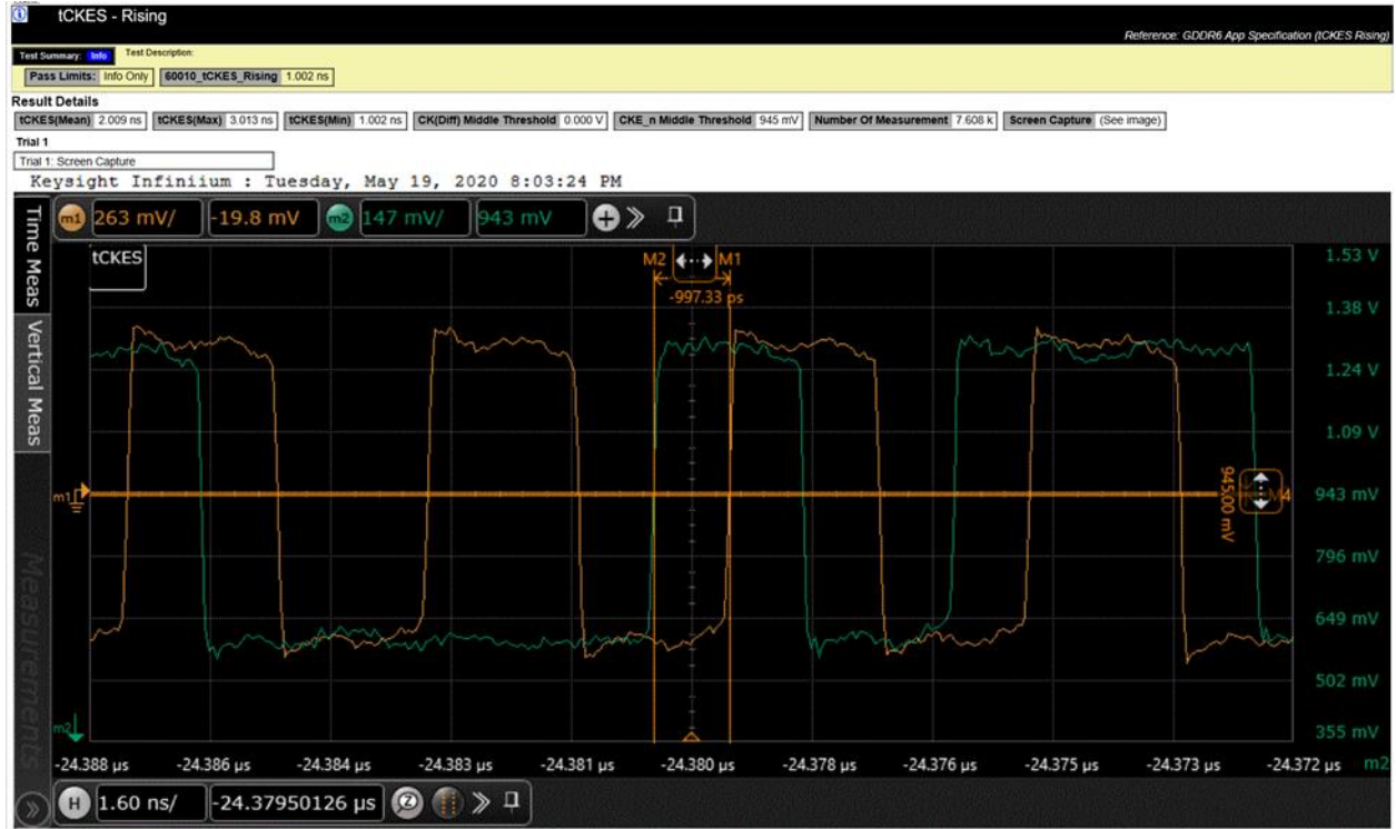
Figure 4. The test application generates a summary report where you can see your device's test results quickly and clearly. Details are available for each test including the test limits, test description and test results, including saved waveforms. In addition, the pass/ fail margin is indicated to give you further insight. Images are included on applicable parameters.
