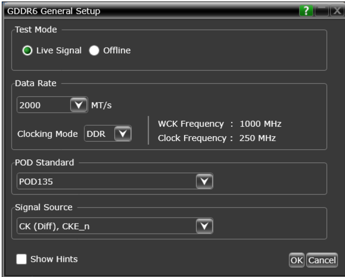
Figure 2. The software provides user-defined controls for test parameters such as voltage threshold values
