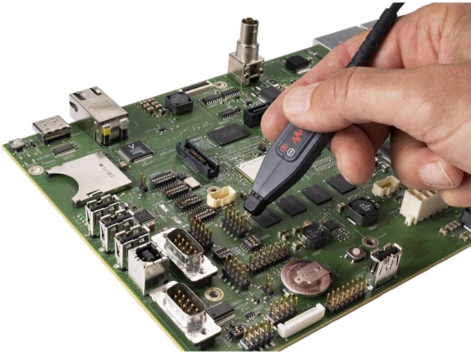
Figure 5. Using the DP001xA Series differential active probe with the adjustable browser probing tip.
