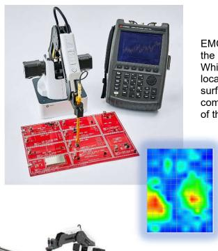
EMC and signal integrity are major concerns in the design of ultra-high speed (>2 GHz) PCBs. While EMScanner allows designers to easily locate emission by placing the PCB on its flat surface, the EMProbe allows users to test the component side of the PCB and adjust the height of the scan.
