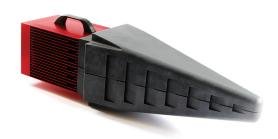
ETS-Lindgren's EMField Generator is a unique, integrated solution for Radiated Immunity testing including IEC/EN 61000-4-3. It combines an amplifier, directional couplers, and an antenna array into one remarkable, simplified design. Nearly all of the generated power is converted into useable field strength.
