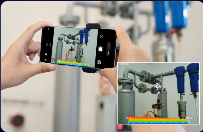
Compressed Air Leak/Vacuum Leak Inspection
