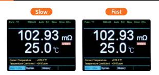
GOM-804/805 has two measurement speed selections, which are Fast reaching 60 readings per second, and Slow 10 readings per second. A major departure from the past, users, in the past, had to juggle between speed and display resolution. GOM-804/805 will not affect resolution despite of any speed selections and will maintain the highest display digits. In other words, reading resolution will not be changed by changing speed and the display digits remain the same.
