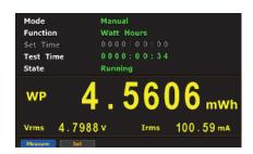
integration at the set time period, and then divide by the time to obtain the average power of the DUT. In addition, when performing integration measurement, GPM-8310 supports automatic level-changing function for the power change of the DUT at different times in order to obtain the most complete integration result within the set time.
