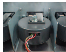
DCCT current sensor (in the PW3337)
