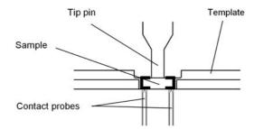
Fig. 1. Sample Electrode and Probes
