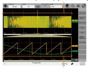
Enlarged display of desired portion of waveform
