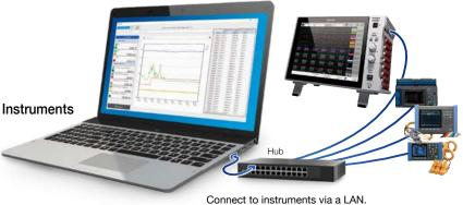
Simultaneous, real-time observation GENNECT One lets you display data from multiple instruments together and in real time in list or graph form.
