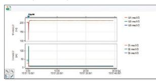
Example voltage dip screen (30 sec. event fluctuation data)
