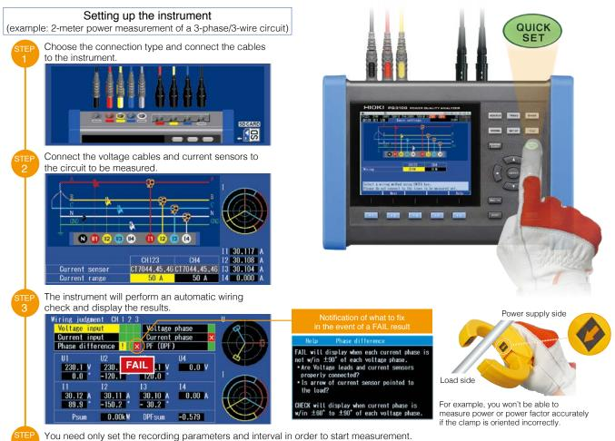
Recording parameters can be set simply by choosing a simple setup preset. (See page 8 for details.)
