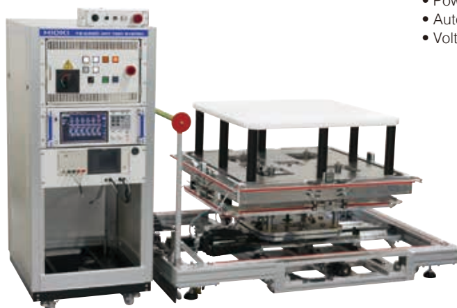
WPT TEST SYSTEM TS2400
