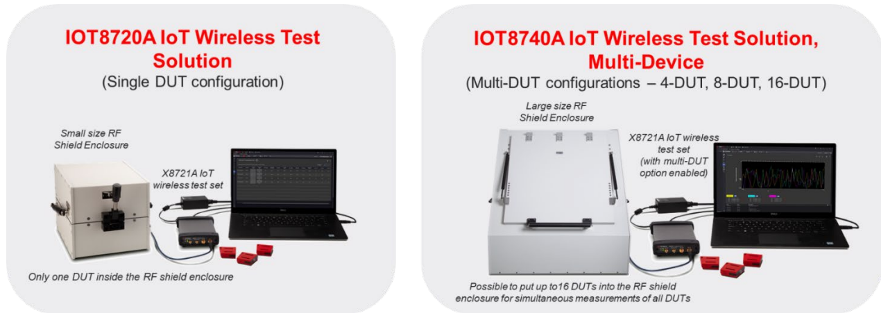
Figure 7. Diagrams showing the single vs multi-device configurations
