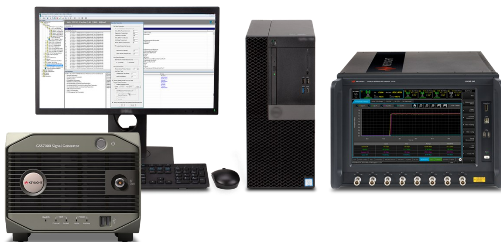
Figure 1. 8100 GNSS OTA test system hardware configuration.
