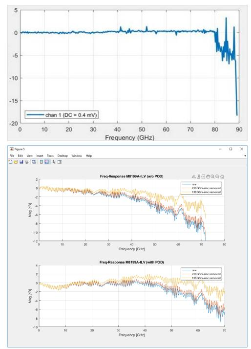
The following graph shows the frequency response after applying digital frequency-response correction up to 80 GHz.
