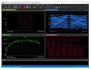
Figure 4. QAM-64, 16 GBaud at 39 GHz carrier
