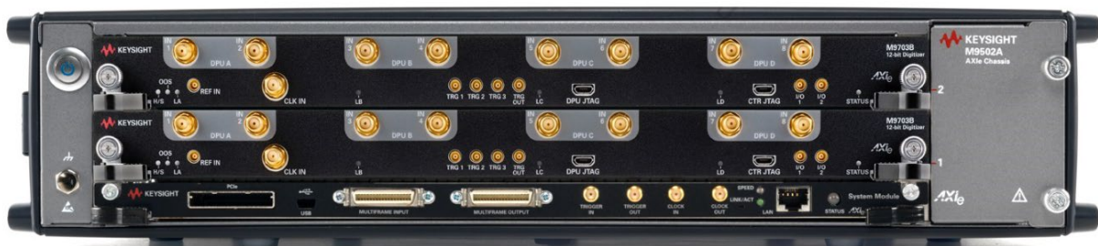
Figure 2. Two M9703B digitizers installed in the M9502A 2-slot chassis, forming a 16-ch 12-bit acquisition system.
