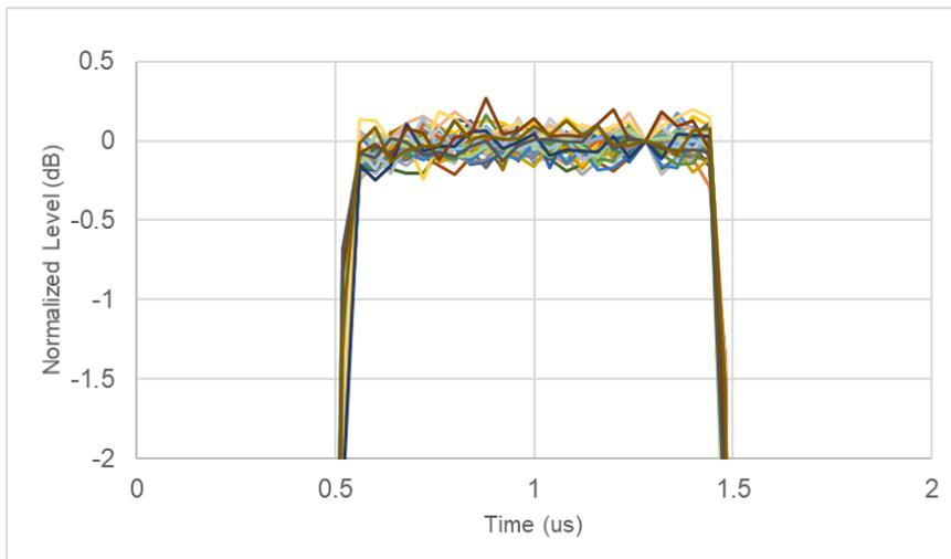
1. Measured with a 500 kHz IF bandwidth, averaging factor of 16 (Average Type = Point). With 1 us pulse width setting. 0.5 u/div.
