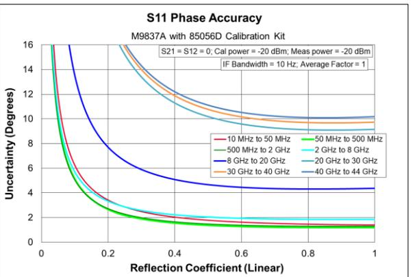
**Table 9. M9834A or M9837A with N4693D Electronic Calibration (ECal) Module with Option 0DC**
