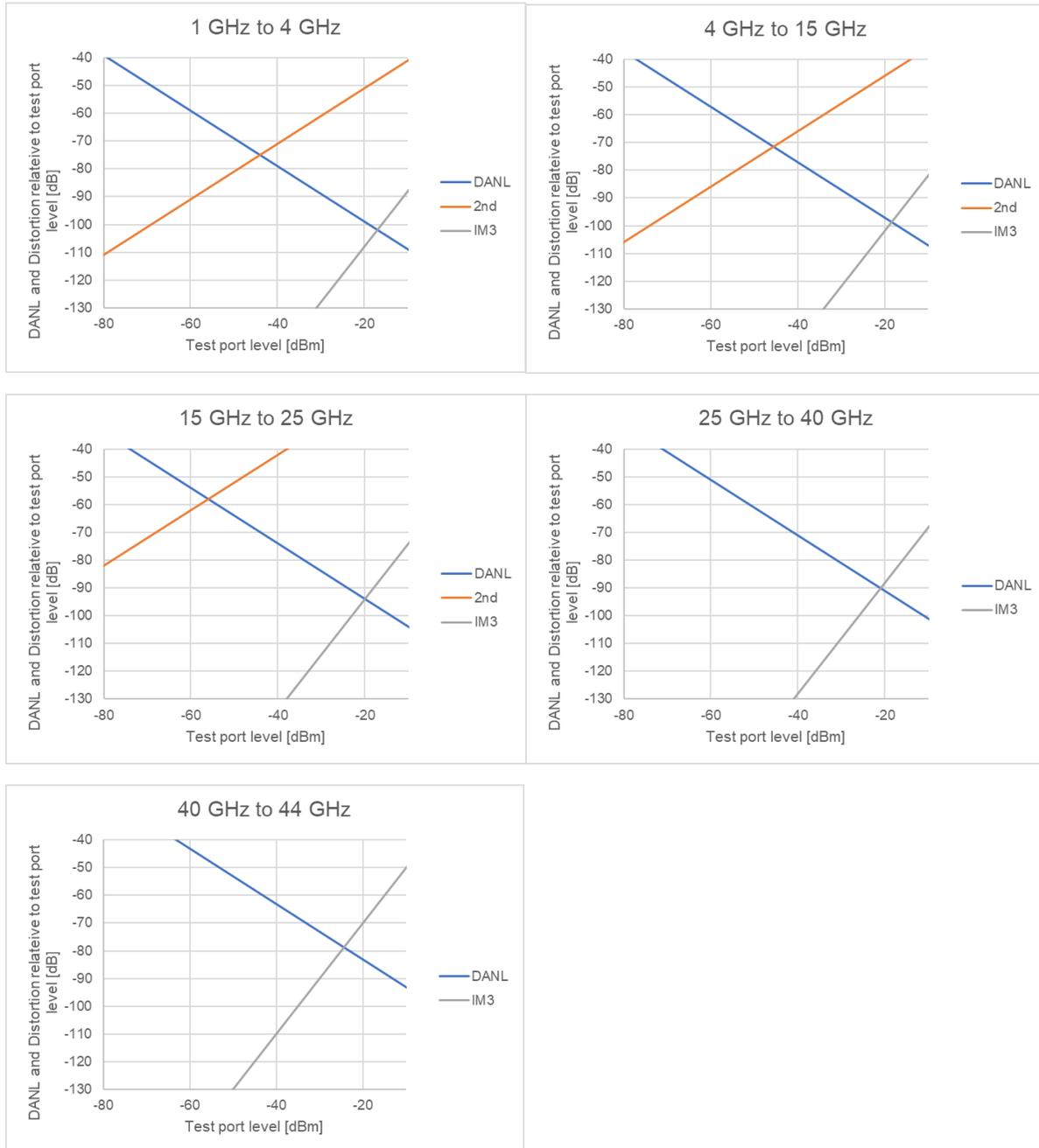
1. With 18 dB Attenuation. 2nd harmonic distortion applies up to 22 GHz
