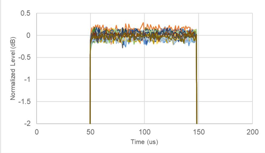
1. Measured with a 500 kHz IF bandwidth, no averaging (Average Type = Point). With 100 us pulse width setting. 50 us/div.
