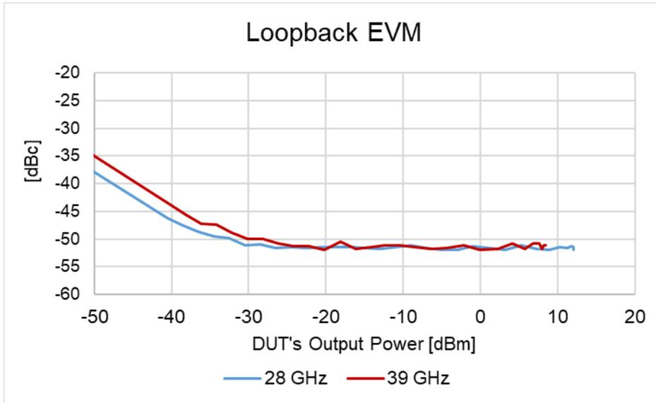
1. Measured ACP & EVM of 11900B adapter (female-female, 2.4-mm connectors) using a compact waveform of 5G NR (32 us period). 100 MHz bandwidth, 64QAM, 60 kHz SCS, 2,979 Number of tones.
