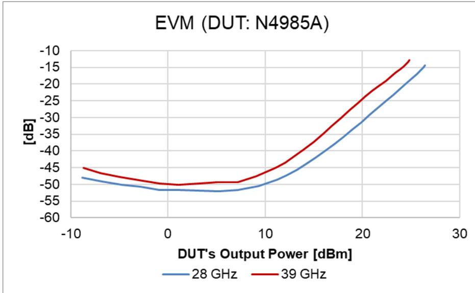
1. Measured ACP & EVM of Keysight N4985A (power amplifier, 2 GHz to 50 GHz with option P25) using a compact waveform of 5G NR (32 us period). 100 MHz bandwidth, 64QAM, 60 kHz SCS, 2,979 Number of tones.
