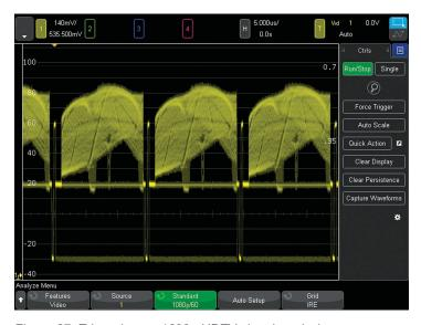
Figure 27. Triggering on 1080p HDTV signal analysis.
