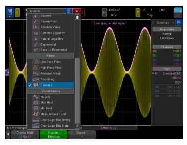
Figure 30. A variety of advanced math functions are standard in the 4000 X-Series.
