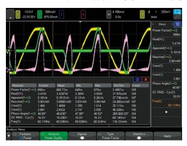
Figure 26. Power quality measurement, one of many in the power measurements application.
