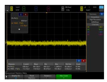
Figure 40. Getting 113 uVrms noise floor at 1 mV/div with the high-resolution mode.
