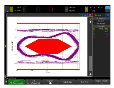
Figure 28. Perform automatic signal quality testing on USB 2.0 low-speed, full-speed, and hi-speed signals.
