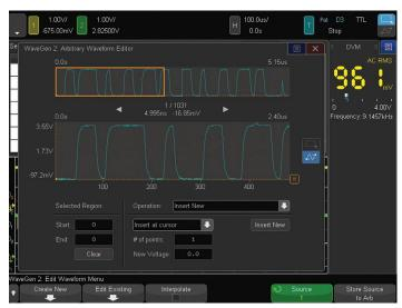
Figure 23. WaveGen arbitrary waveform editing screen.
