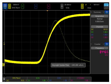
Figure 3. The 4000 X-Series captures a glitch occurring once in a million waveform cycles.
