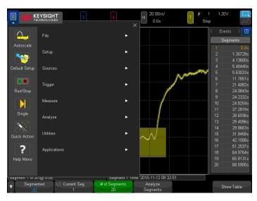
Figure 14. Use the Keysight pull-down menu for Window-like operation.
