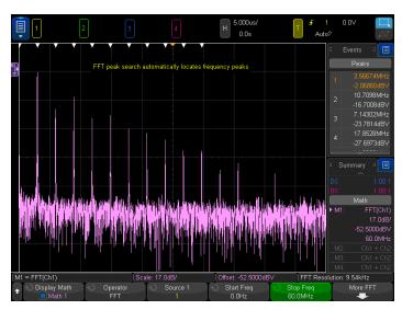
Figure 10b. The 4000 X-Series was set up to capture clock signals for FFT analysis ☐ Using the search and navigation capability, the scope found, marked (white triangles) and quickly navigated to the first 11 frequency peaks occurrences. You can sort it in the order of frequency or amplitude.
