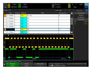
Figure 11. Using the error condition search, the 4000 X-Series quickly found 5 places with a missing acknowledgment in an I<sup>2</sup>C serial bus. The navigation feature moves between the errors and zooms automatically to show the error packet.
