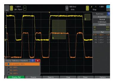
Figure 33. Store and recall up to four reference waveforms.
