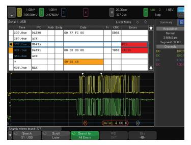
Figure 21. USB 2.0 trigger, decode and "lister" display.
