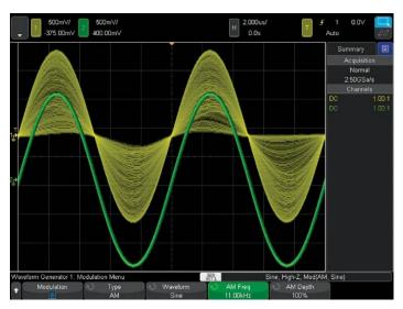
Figure 22. WaveGen sine wave output with and without added AM modulation.
