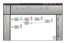
The graphical signal processing interface makes it easy to setup and display math functions and other types of simulations.
