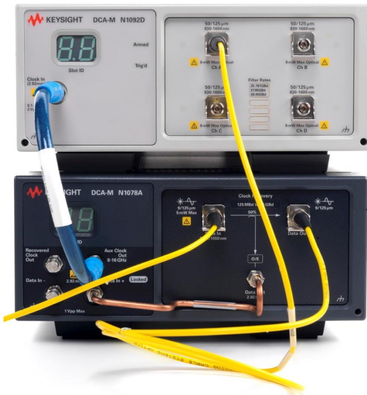
N1078A Clock Recovery triggering a N1092D DCA-M
