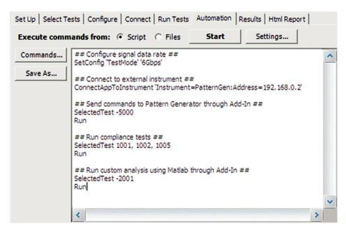
Figure 10. Remote Programming script in the Automation tab.
