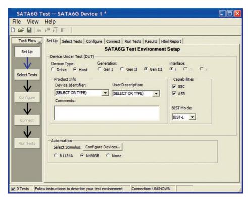
Figure 1. The Keysight SATA software setup tab allows you to choose the interface type of your product and the relevant test speed, then automatically configures the measurements and limits appropriately for your specific product per the specification requirements.
