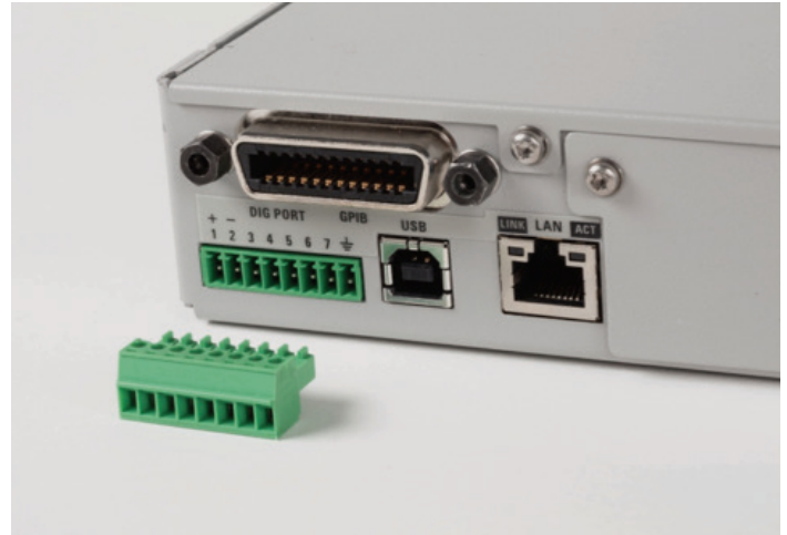
Figure 5. Digital control port on rear panel.
