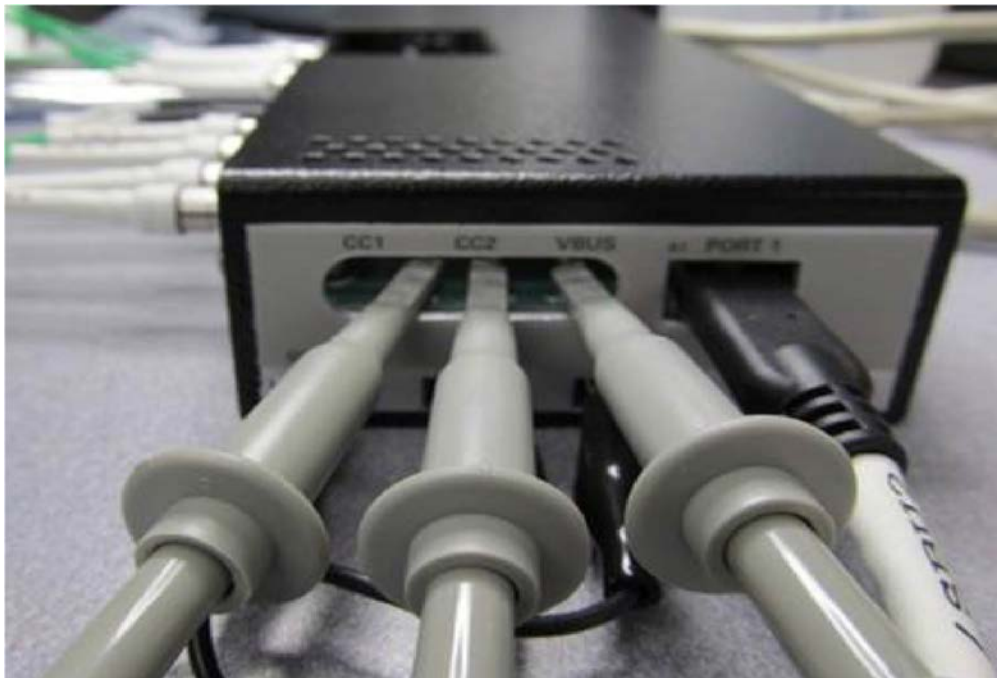
Figure 11. VBus probing on N7018A.
