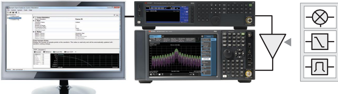
Figure 1. Typical component test configuration using Signal Studio with an X-Series signal generator and analyzer.
