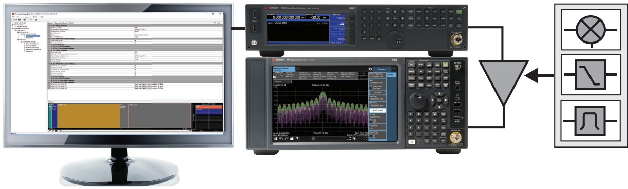
Figure 1. Typical component test configuration using Signal Studio's basic capabilities with a Keysight X-Series signal generator and an X-Series signal analyzer
