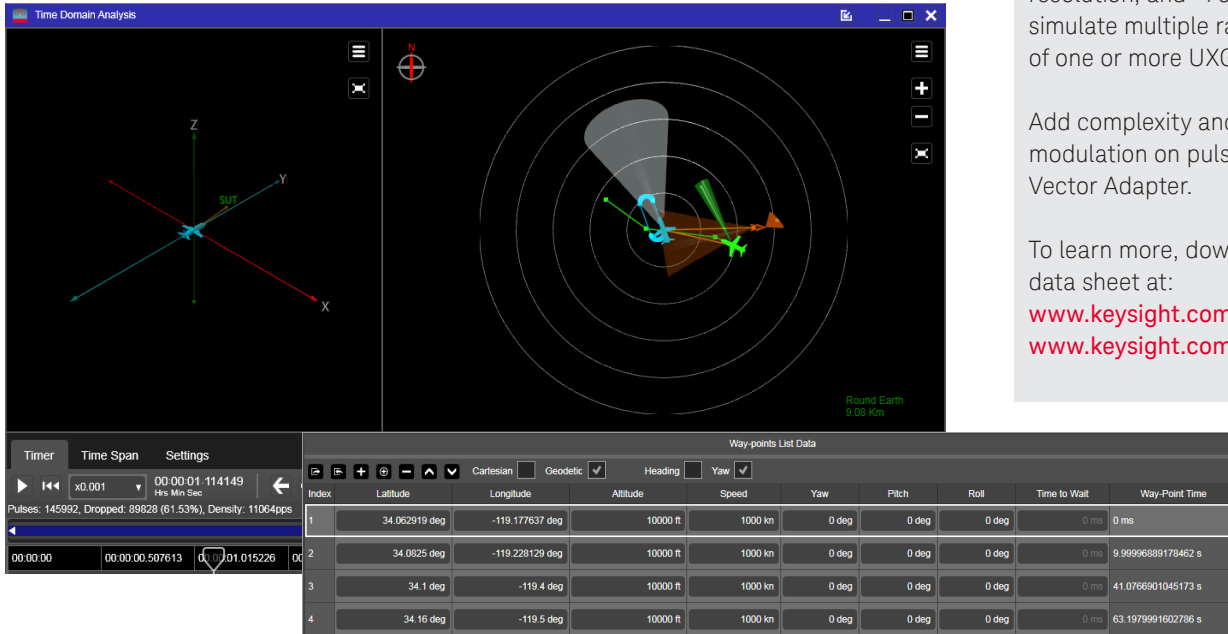
Figure 5. Import waypoints to define flight path for SUT or environment threats.
