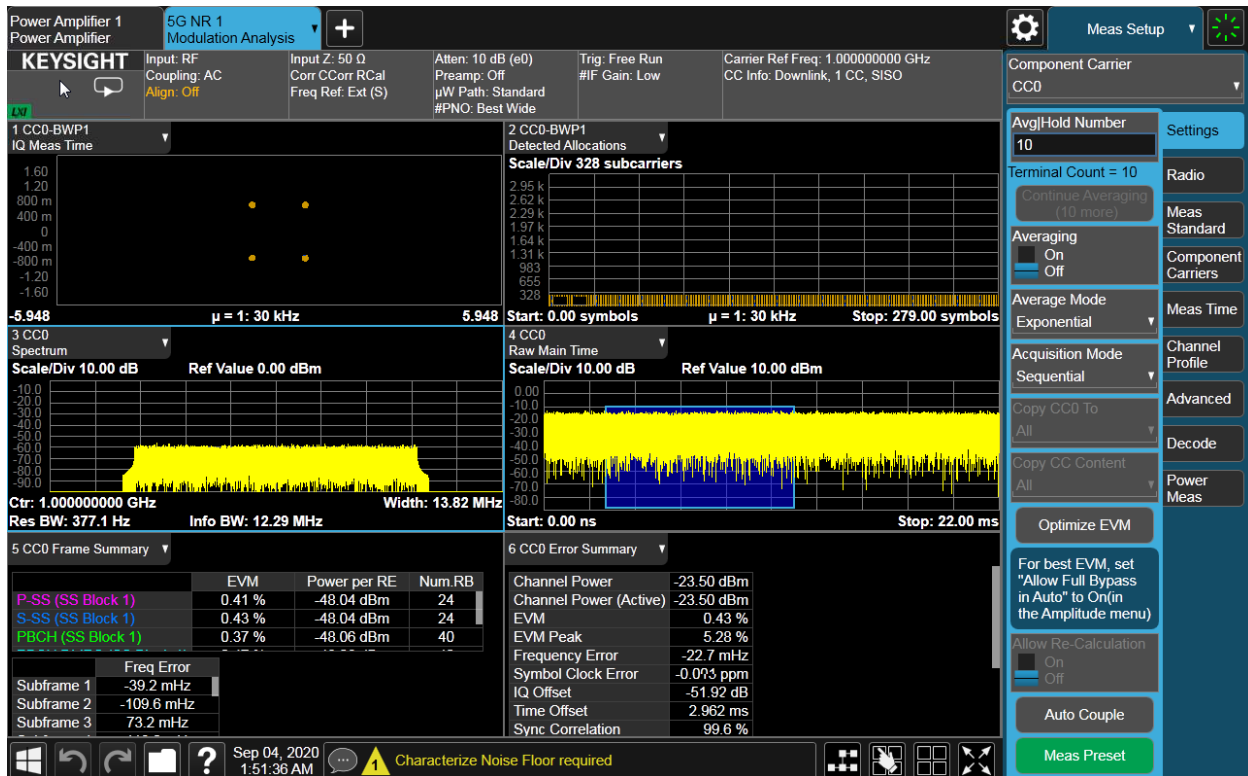
Figure 8. Switch from PA Test mode to 5G NR mode to check the correct demodulation settings
