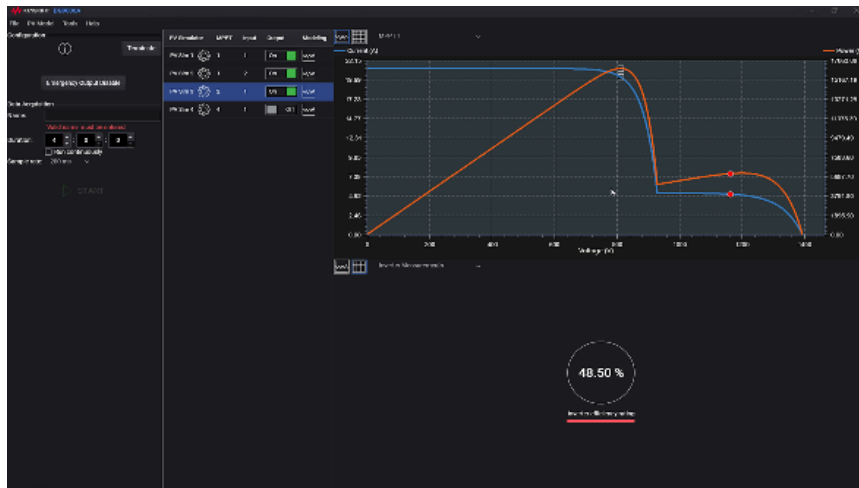
Figure 5. DG9000A MPPT efficiency
