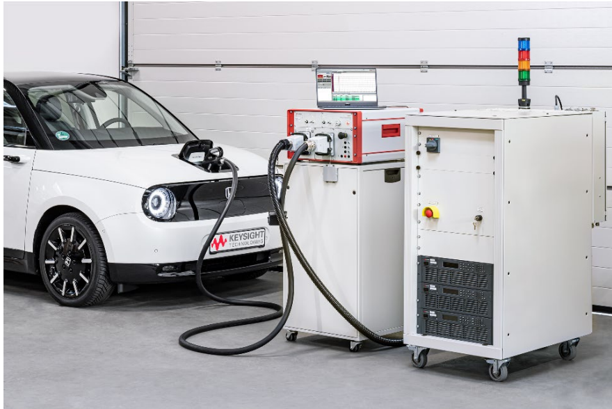
Figure 7. AC charging test with SL1201A AC Emulator and SL1040A Charging Discovery System test.
