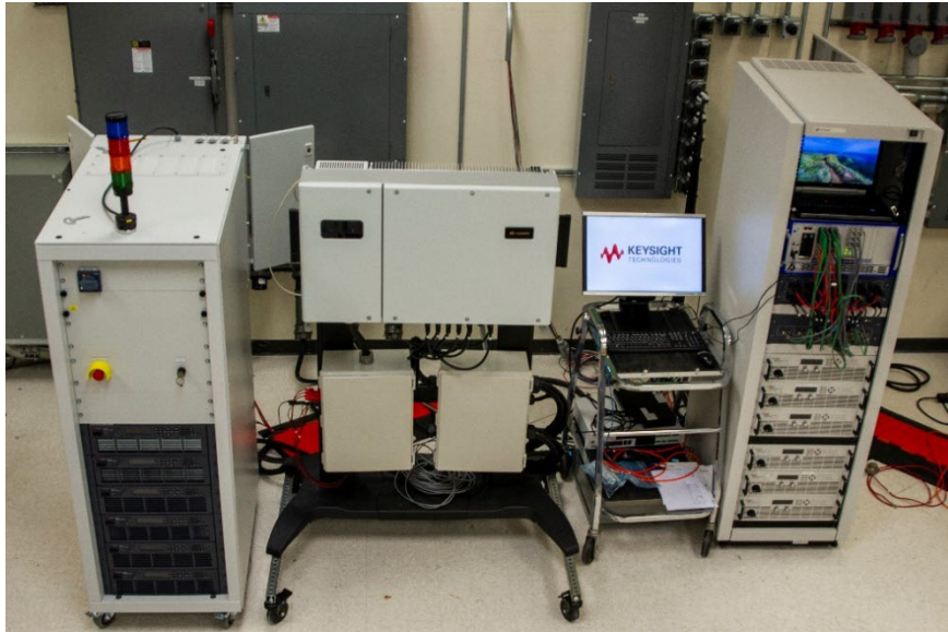
Figure 5. SL1202A AC Emulator with PV8900A Solar Array Simulators and DG9000A PV software.
