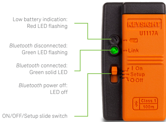
Figure 4. The U1177A as illustrated
