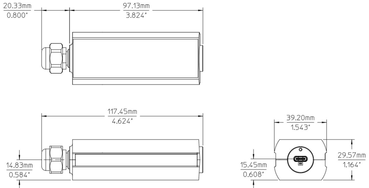
**Figure 8.** Mechanical dimension of U1833B
