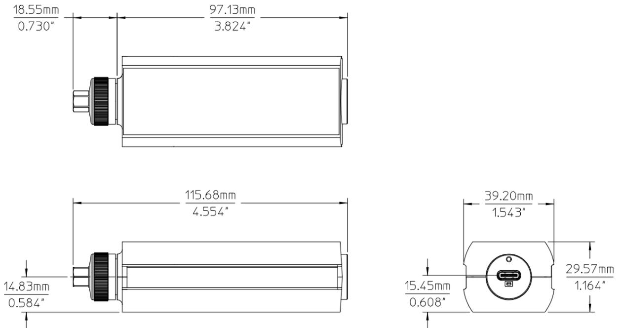
**Figure 10.** Mechanical dimension of U1833C
