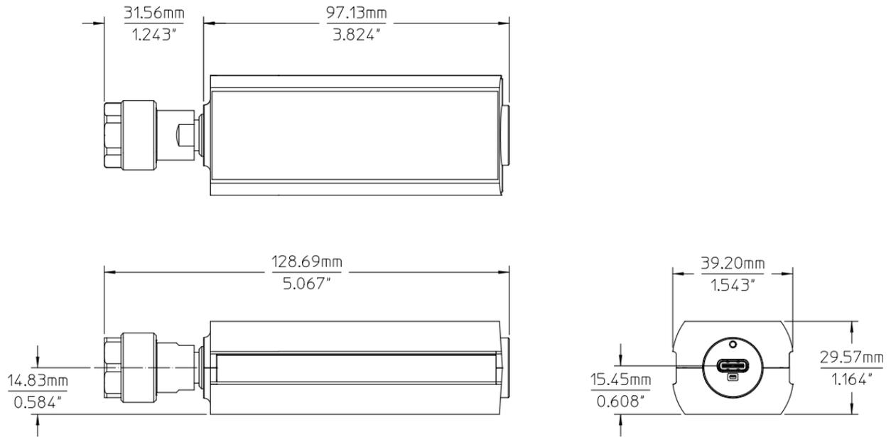
**Figure 7.** Mechanical dimension of U1833A
