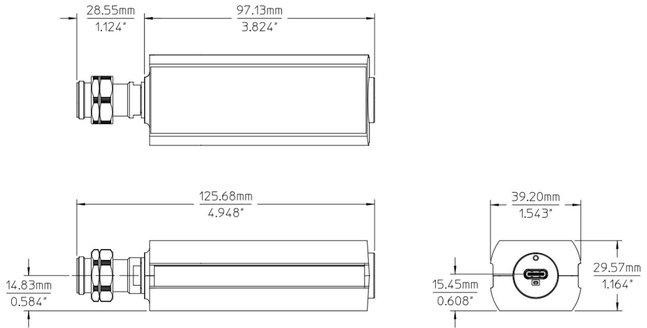
**Figure 11.** Mechanical dimension of U1833D
