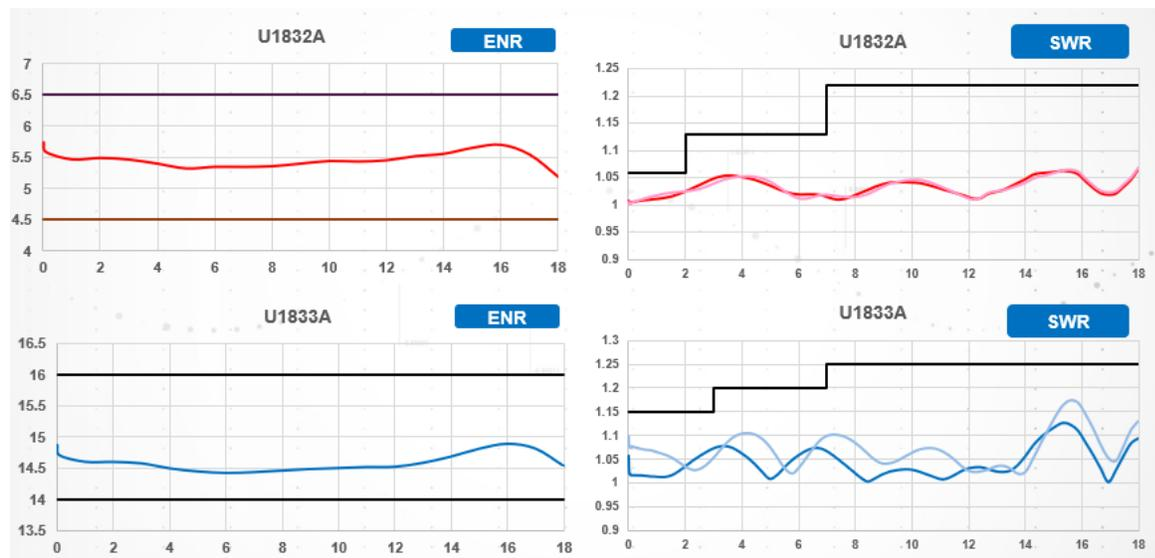
Figure 1. Typical ENR and return loss of U1832A and U1833A
