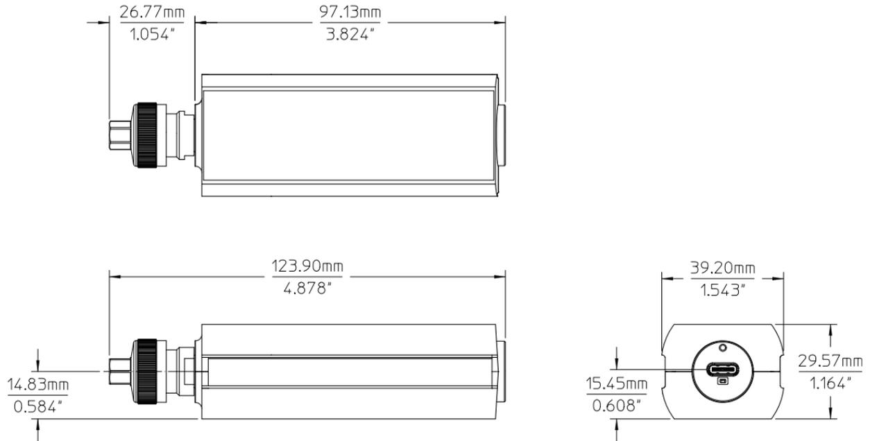
**Figure 9.** Mechanical dimension of U1832C
