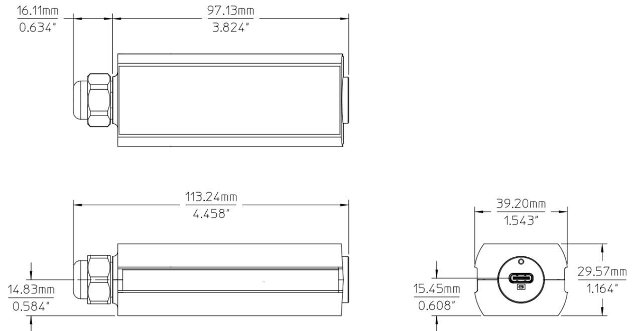
**Figure 6.** Mechanical dimension of U1832B
