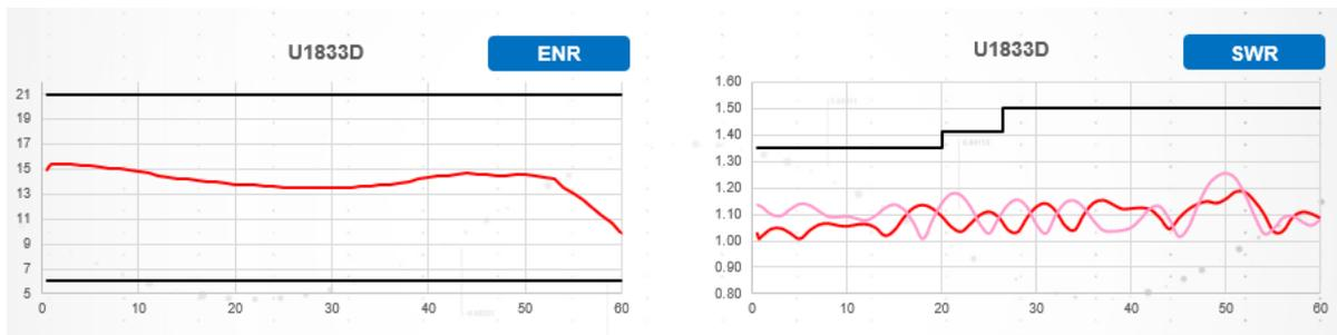
Figure 4. Typical ENR and return loss of U1833D
