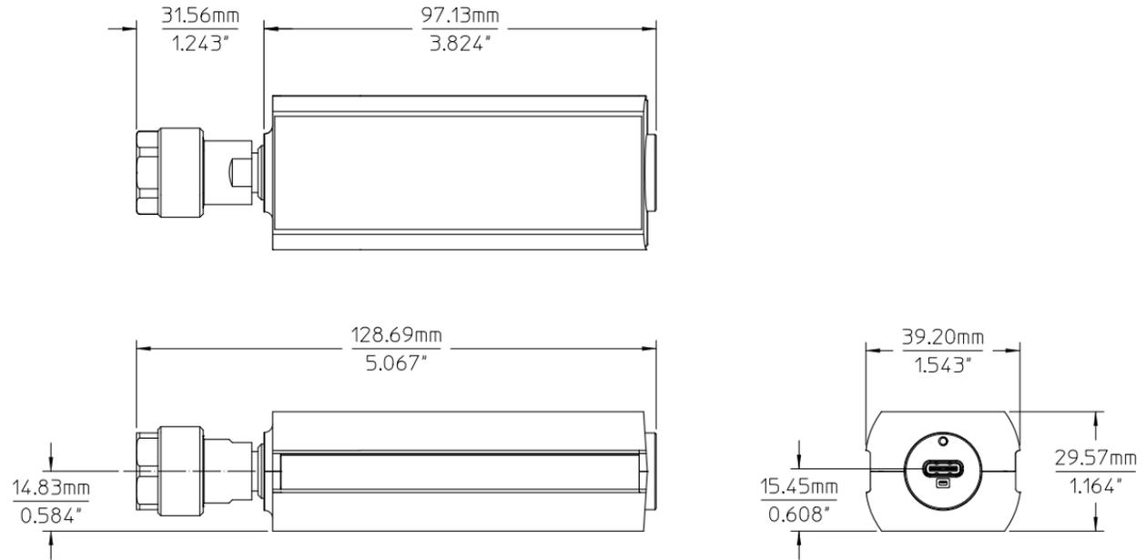
**Figure 5.** Mechanical dimension of U1832A
