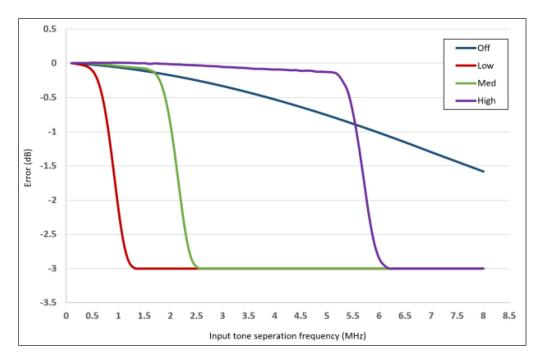
Figure 8. U2063/64/65 and L2061/62/63/64/65XA error in peak-to-average ratio measurements for a two-tone input (High, Medium, Low and Off video bandwidth settings).
