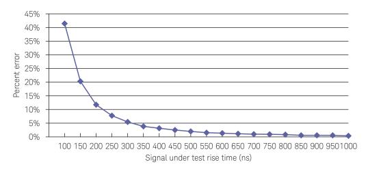
Figure 6. Measured rise time percentage error versus signal under test rise time.
