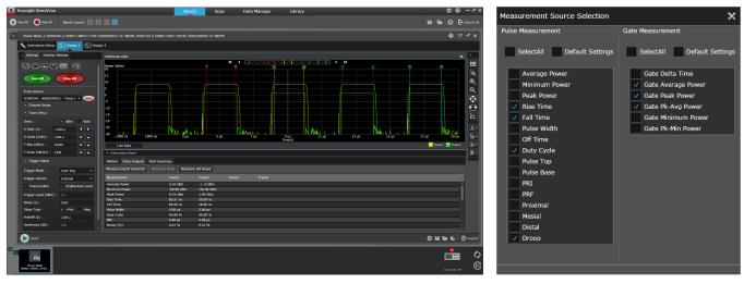
Figure 10. Multi-channel trace display with 4-pairs of gates and automatic pulse parameters measurement (sample screen shot with two U2042XAs).
