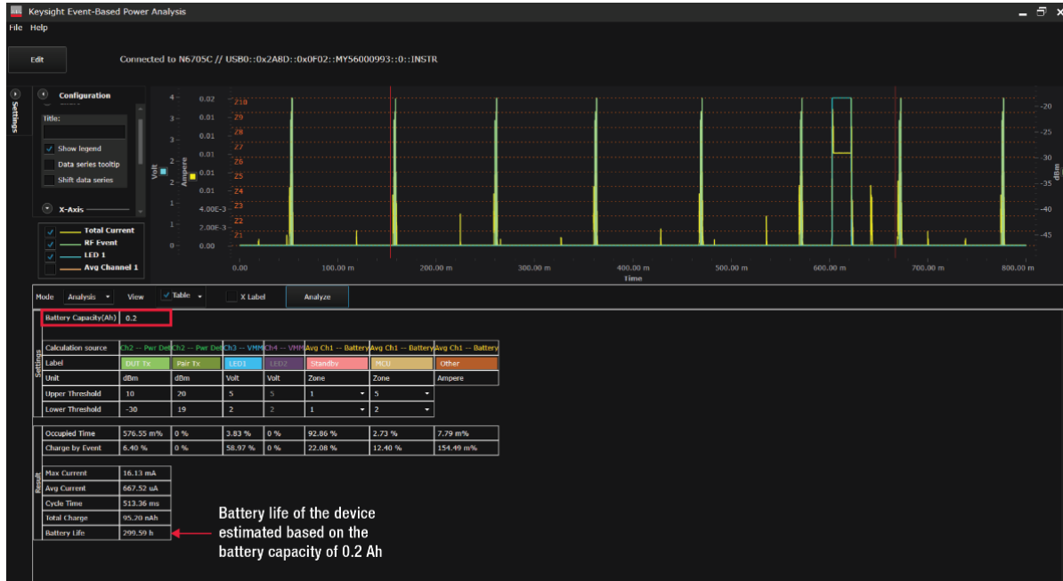
Figure 10 - Battery life predicted based on five full operational cycles and 0.2-Ah battery capacity
