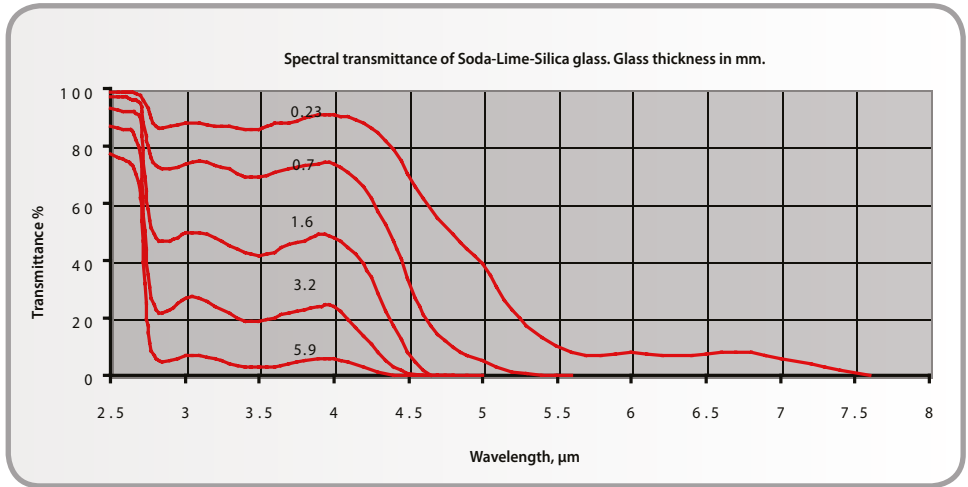
Figure 5. Transmission curves for a common industrial glass in five thicknesses from 0.23 to 5.9mm
