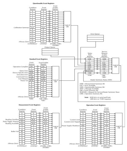
\*Note: URQ indicates that the "Lock" key on the panel has been used. (Entering lock from unlock or Entering unlock from lock).
